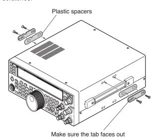
Once the bracket is installed onto the vehicle, prepare the transceiver by loosely screwing in the rear screws. Hook those screws onto the rear guide rail of the mounting bracket then adjust the transceiver to your desired angle before tightening the screws. Insert and tighten the front screws to secure the transceiver in place.
