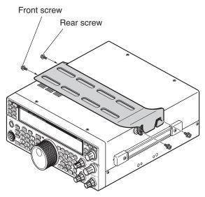
To remove the transceiver from the bracket, first remove the front screws, then loosen the rear screws slightly and pull the transceiver forward to unlatch it from the bracket.
