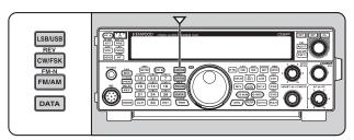
Access Menu No. 23 then press [M.IN] to select "on" to turn the Auto Mode selection ON. When it is ON, "AUTO" appears. As a default, if you change the frequency above or below 9.5 MHz, the transceiver automatically switches modes; LSB for frequencies under 9.5 MHz and USB for frequencies 9.5 MHz and over. You can further add the frequency borders to the Auto Mode selection {page 51}.
